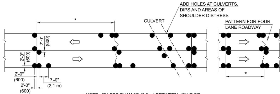
\* NOTE: IF LESS THAN 20' (6.0 m) BETWEEN JOINT OR CRACKS USE 2 HOLES AT CRACK AS CIRCLED.
