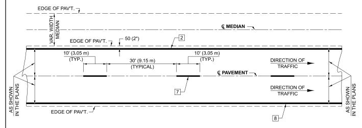
NOTE: PAVEMENT MARKINGS ARE TO BE EXTENDED THROUGH OMISSIONS WHEN APPLICABLE. NOTE: SEE ARTICLES 780.04 & 781.03 FOR LOCATION OF STRIPES AND MARKERS RELATIVE TO EDGES OR JOINTS.
