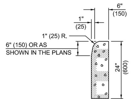
TYPICAL DETAIL OF CONCRETE CURB, TYPE B (SPECIAL)
