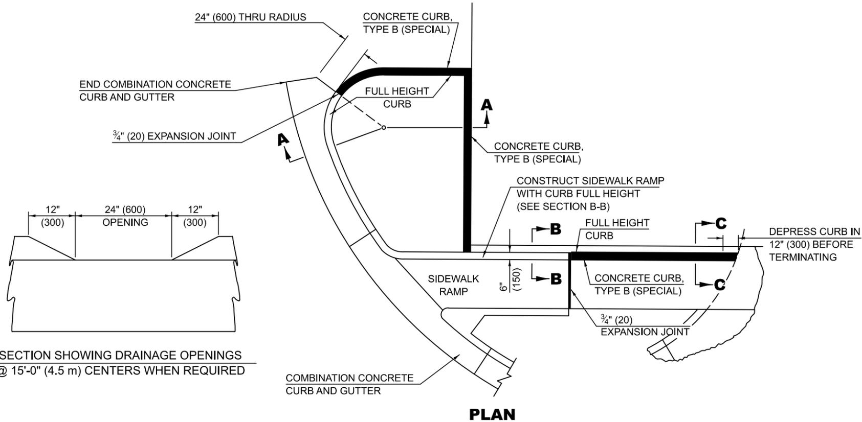
SECTION SHOWING DRAINAGE OPENINGS @ 15'-0" (4.5 m) CENTERS WHEN REQUIRED
