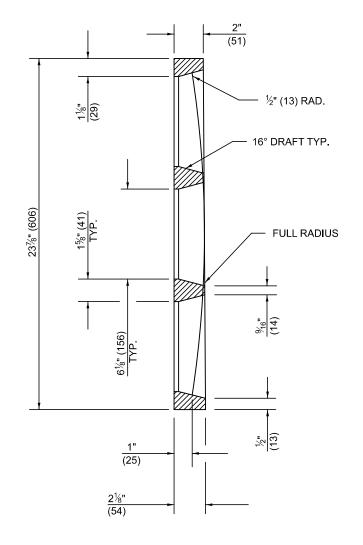
MATERIAL: CAST GRAY IRON ASTM A-48, CLASS 35B
