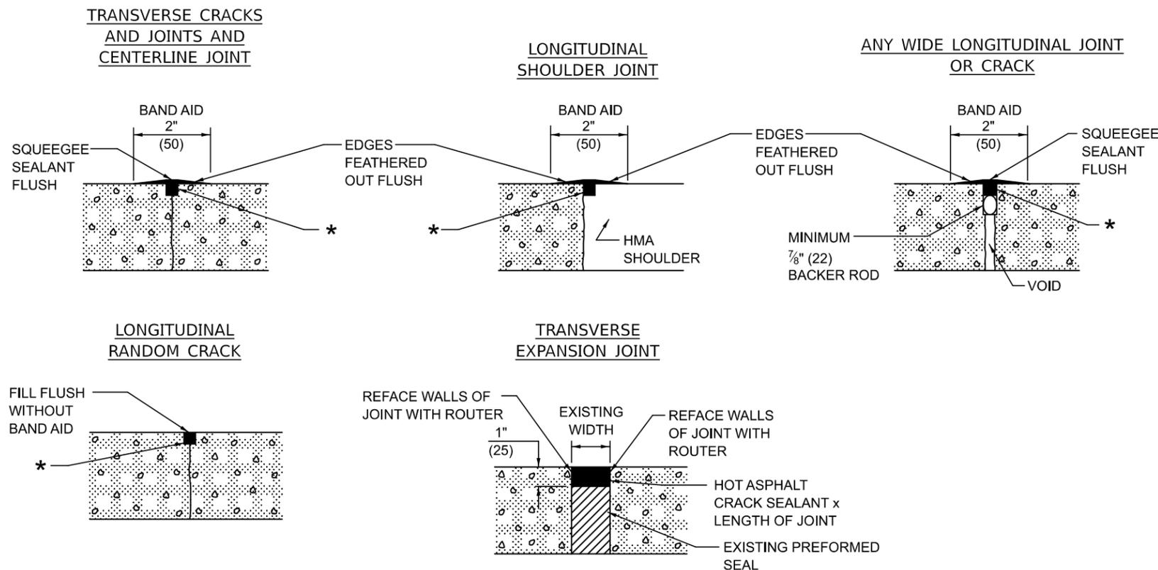
\* HOT ASPHALT CRACK SEALANT
