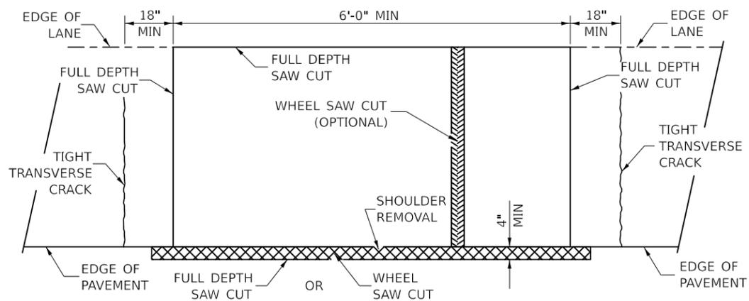
**PAVEMENT SAWING DETAIL
