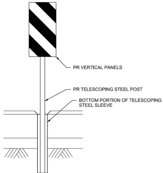
NOTE: FOR INSTALLATION OF VERTICAL PANELS IN AREAS OF CROSSOVER PAVEMENT, 3" Ø HOLES SHALL BE CORED THROUGH PAVEMENT FOR PLACEMENT. TELESCOPING STEEL POLES SHALL BE PLACED 1" BELOW SURFACE AS SHOWN, AND WORK SHALL BE DONE TO THE SATISFACTION OF THE ENGINEER. WHEN OPENING CROSSOVER, PANELS SHALL BE REMOVED AND HOLES SHALL BE LEFT IN PLACE. COST OF PANELS, POSTS, SLEEVES, TYPE III BARRICADES, SIGNS, AND CORING SHALL BE INCLUDED IN TRAFFIC CONTROL AND PROTECTION.
