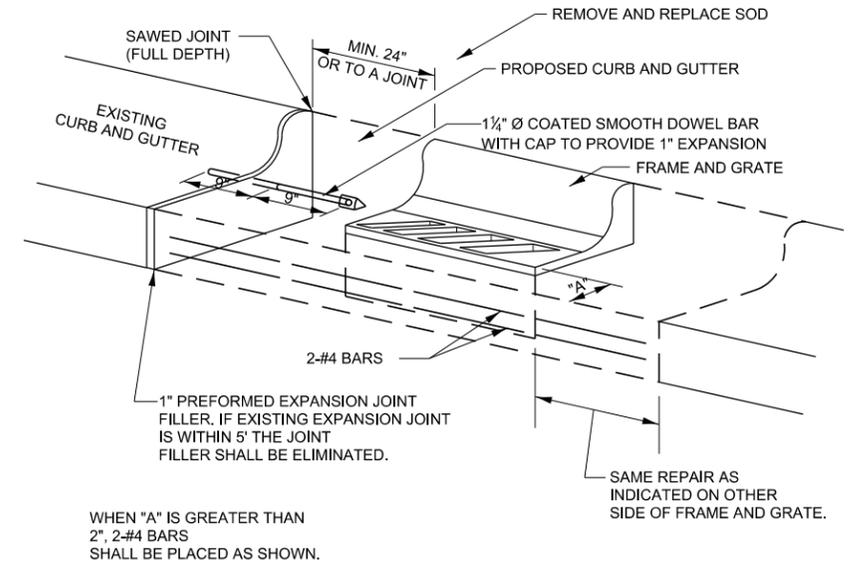
**DETAILS FOR CURB & GUTTER REPLACEMENT
