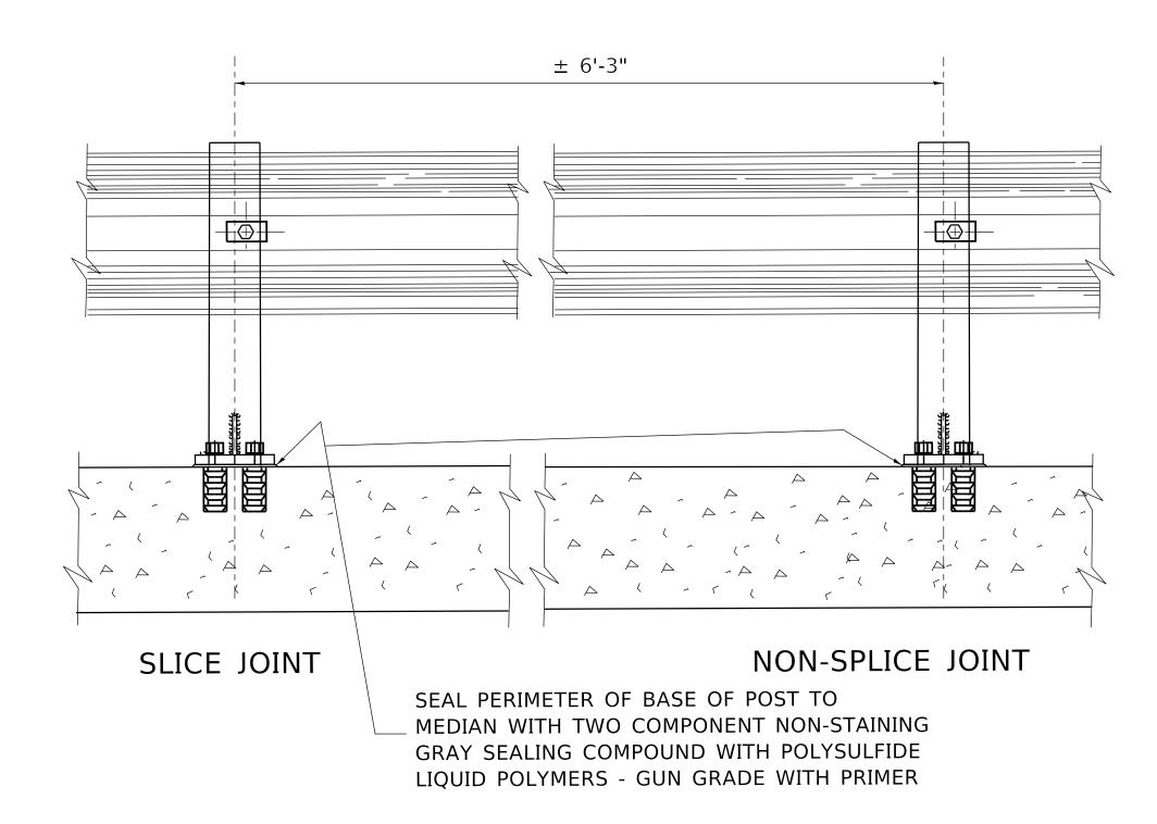
NOTE: DIAMOND TIPPED DRILL SHALL BE USED TO DRILL THRU REINFORCEMENT BARS
