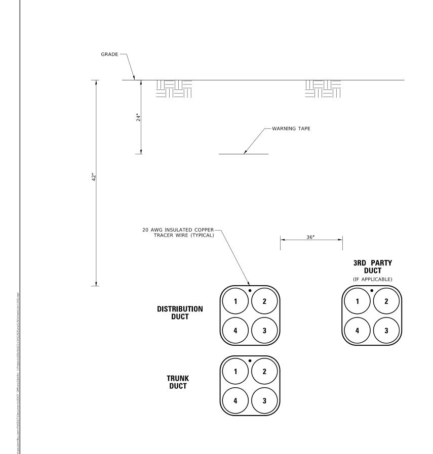
DISTRIBUTION DUCT MICRODUCT CELL ASSIGNMENTS
