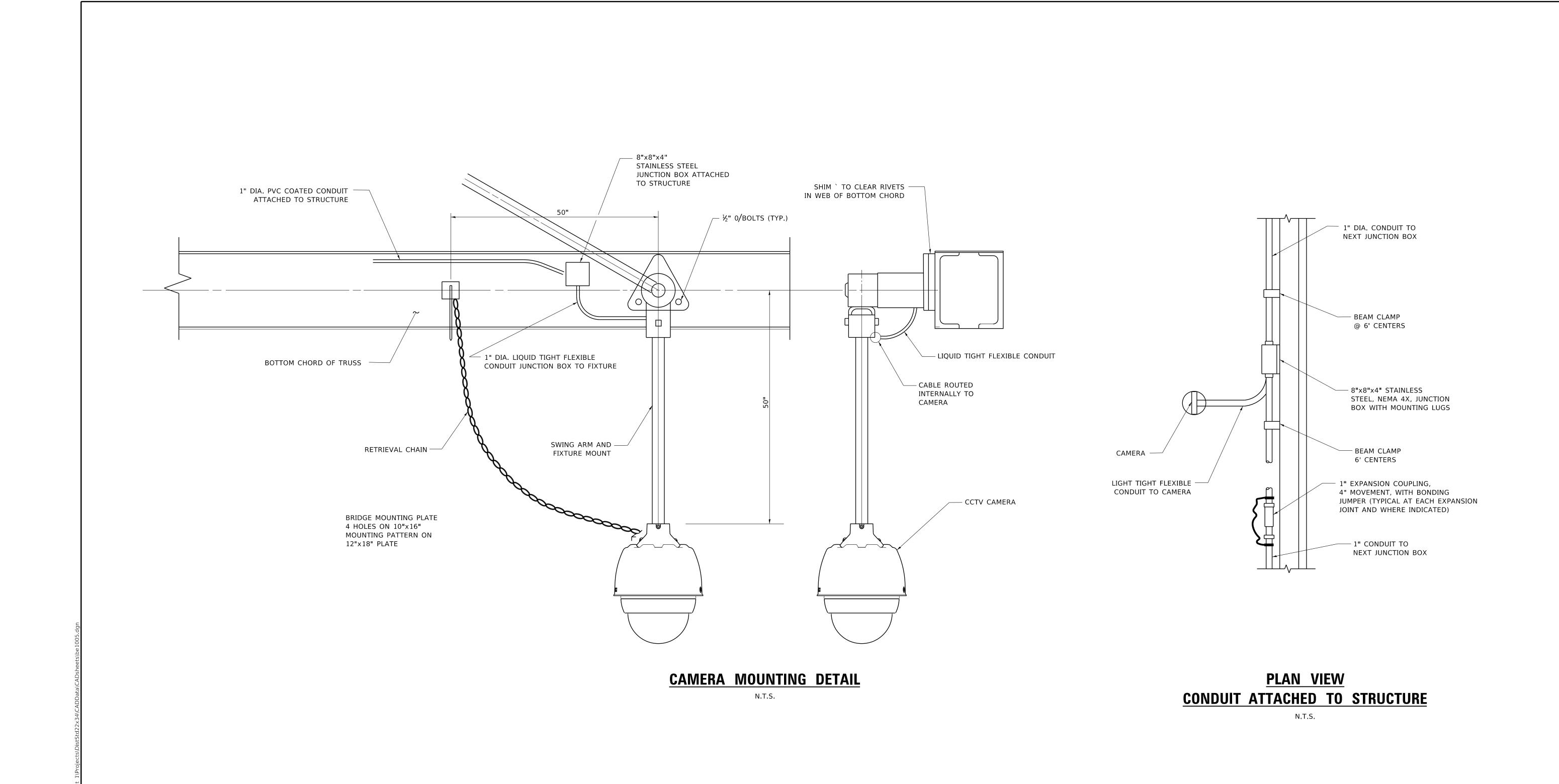
BE-1005 COUNTY TOTAL SHEET NO. DESIGNED -REVISED - 04-23-10 USER NAME = footemj SECTION **BRIDGE MOUNTED** STATE OF ILLINOIS REVISED DRAWN **CCTV CAMERA** REVISED -**DEPARTMENT OF TRANSPORTATION** CHECKED -PLOT SCALE = 50.0000 ' / in. CONTRACT NO. BE-1005 OF 1 SHEETS STA. REVISED -DATE PLOT DATE = 4/22/2019SCALE: NONE SHEET 1 TO STA. ILLINOIS FED. AID PROJECT
