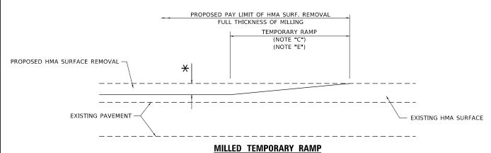
(FOR BUTT JOINT AND HMA TAPER SEE DETAIL BELOW)
