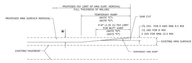
HMA CONSTRUCTED TEMPORARY RAMP
