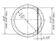
1"  $\oslash$  LADDER RUNG, TYPE "X", LENGTH 2'-11" OR 3'-4" INSERTED INTO 2 O HOLE IN WALL & PLUGGED BY MANUFACTURER WITH NON-SHRINKING GROUT.
