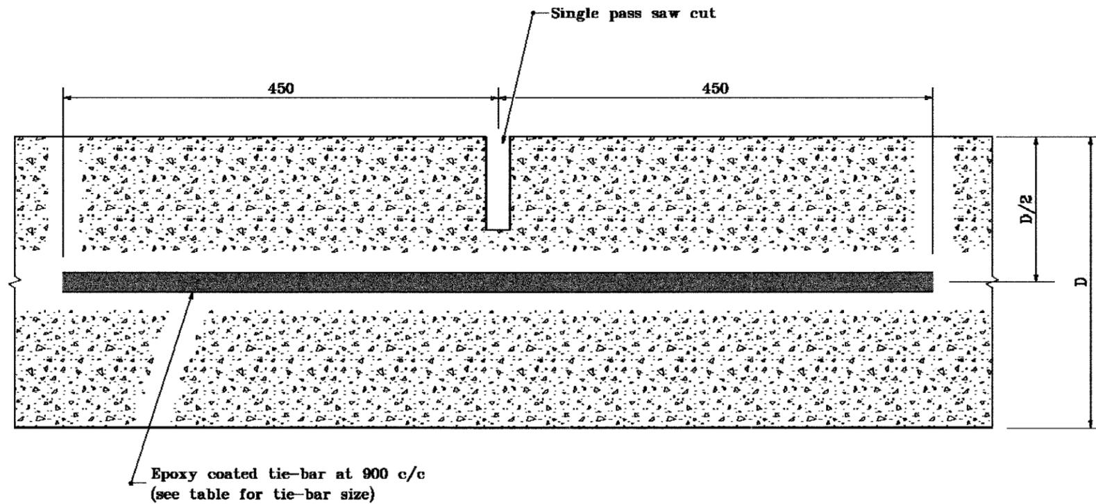
**TRANSVERSE SECTION THROUGH CONCRETE PCCP**
