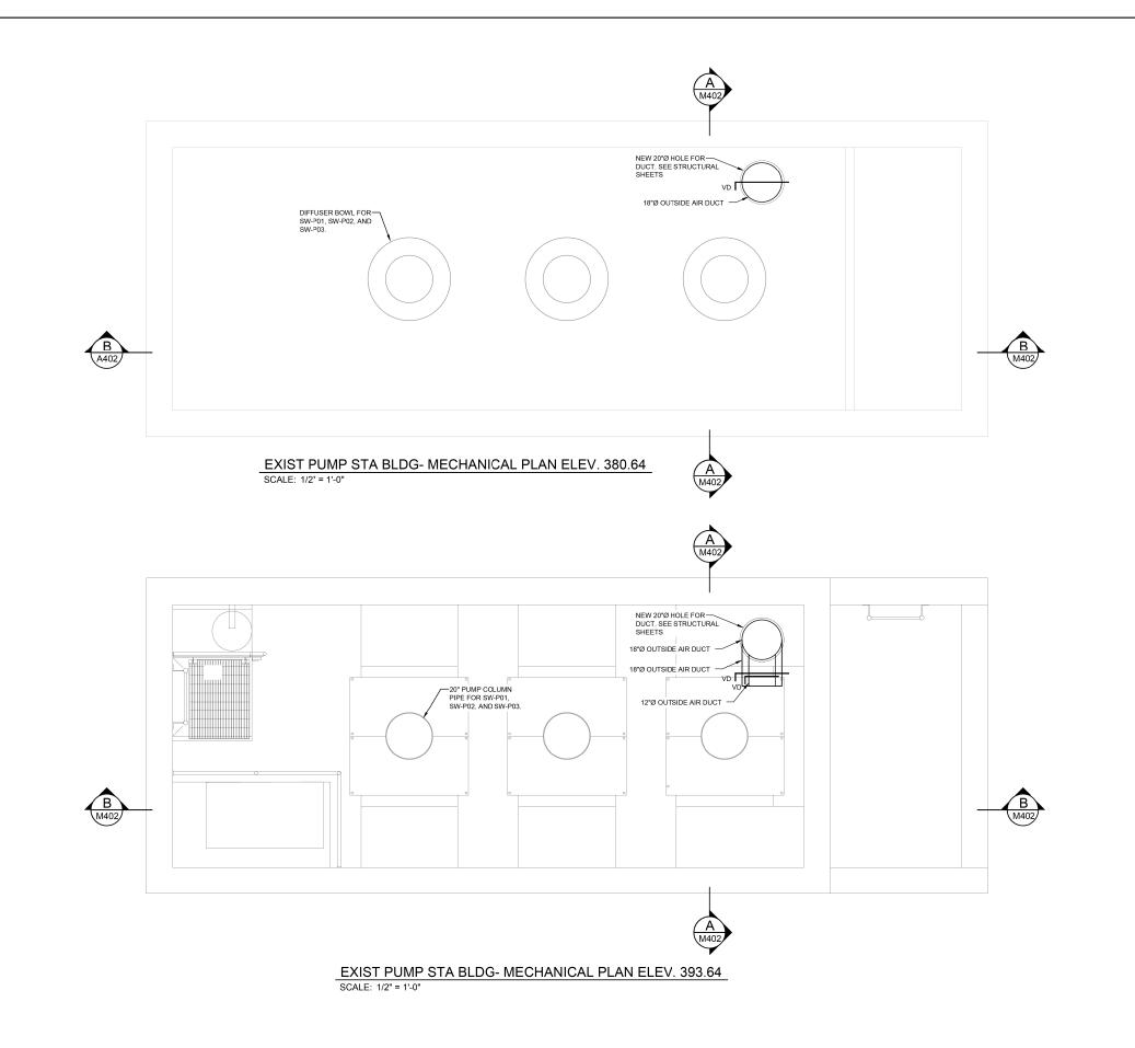
THE STORMWATER PUMP STATION ELECTRICAL CLASSIFICATION IS CLASS 1, DIVISION 2, GROUP D. ALL EQUIPMENT INSTALLED AND INSTALLATION METHODS WITHIN OR ON THE STORMWATER PUMP STATION SHALL BE SUITABLE FOR THIS CLASSIFICATION.
