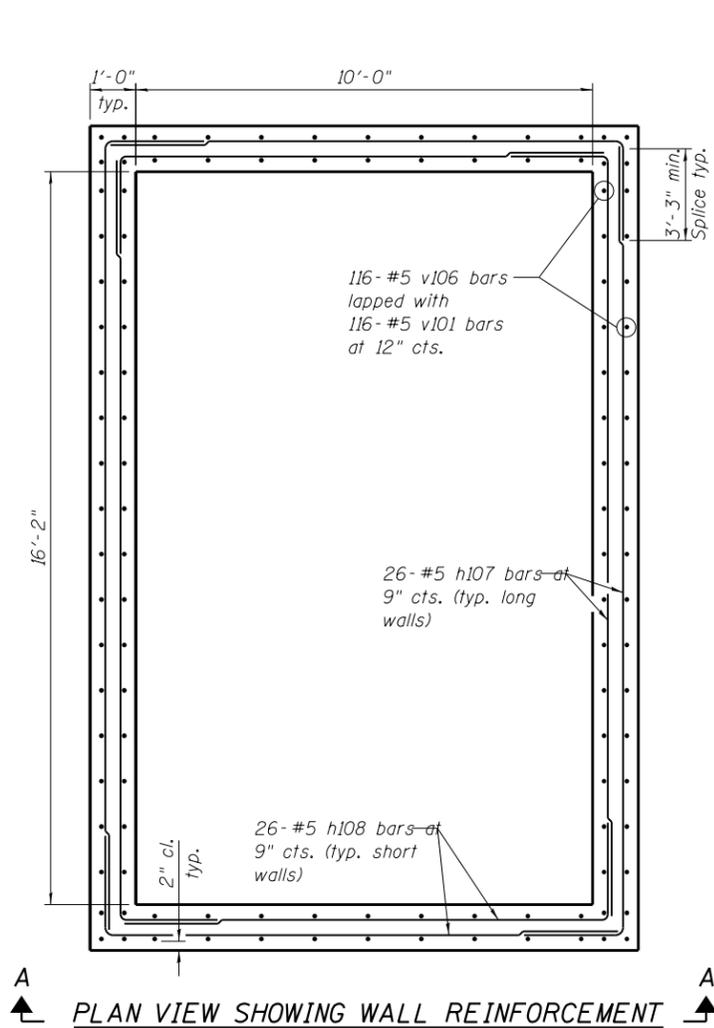
PLAN VIEW SHOWING WALL REINFORCEMENT
