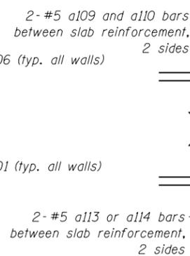
TYPICAL ADDITIONAL REINFORCEMENT AROUND MANHOLE FRAME LID
