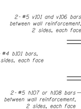
TYPICAL ADDITIONAL REINFORCEMENT AROUND PIPE PENETRATIONS
