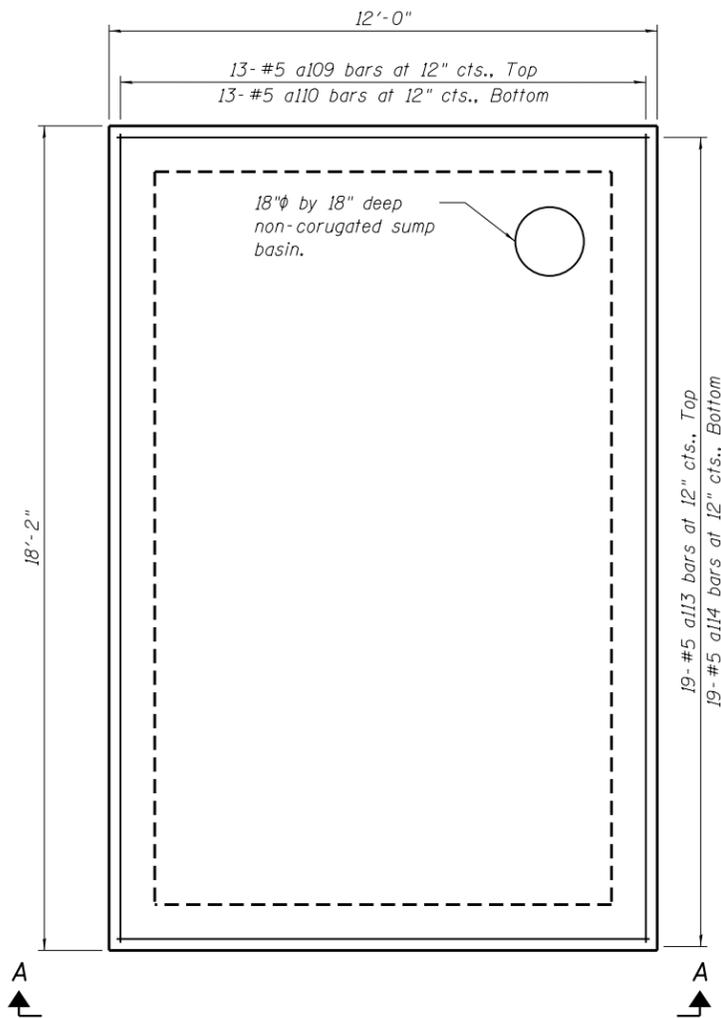
PLAN VIEW SHOWING FOOTING REINFORCEMENT
