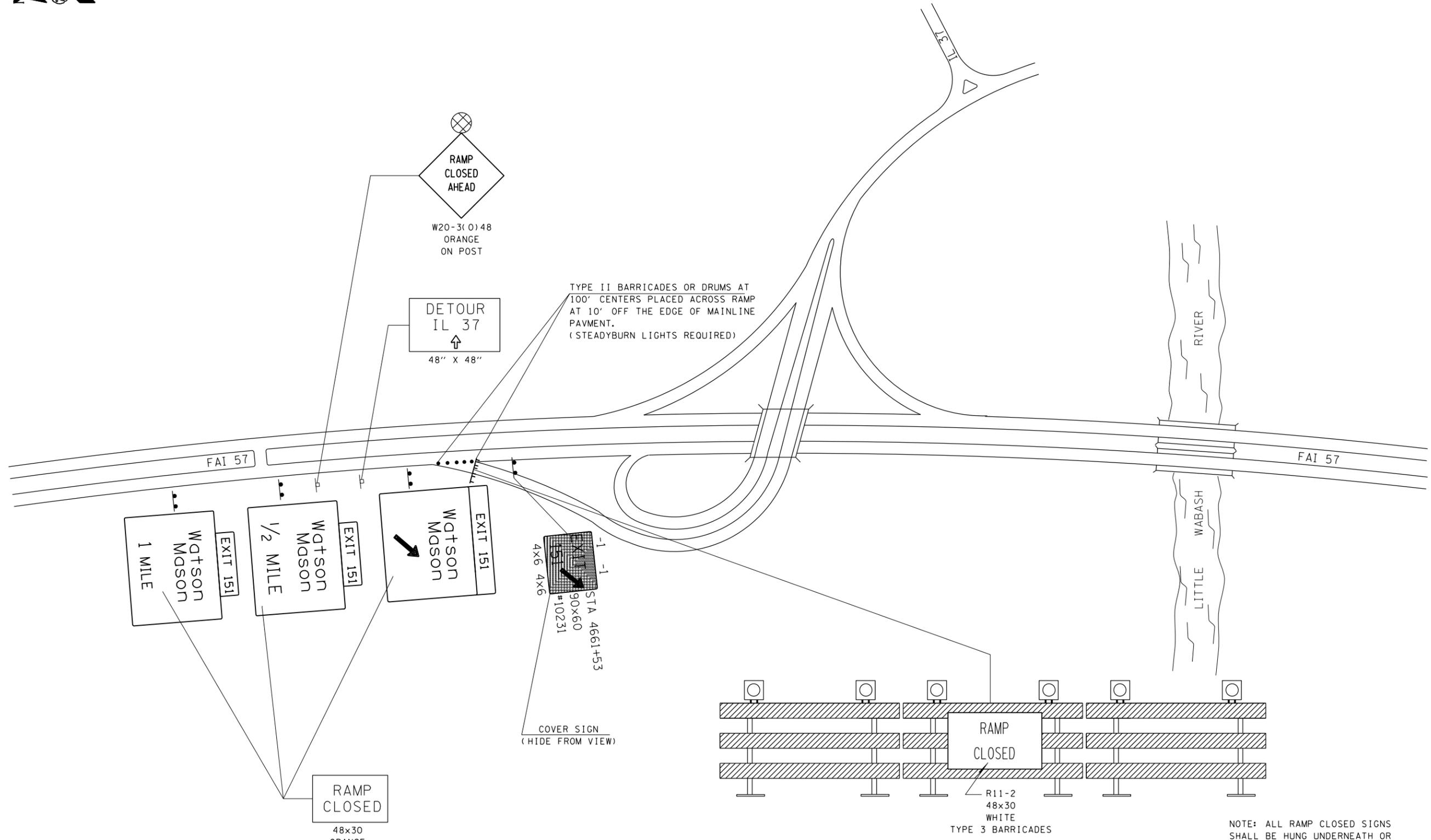
TYPE II BARRICADES OR DRUMS AT 100' CENTERS PLACED ACROSS RAMP AT 10' OFF THE EDGE OF MAINLINE PAVEMENT. (STEADYBURN LIGHTS REQUIRED)
