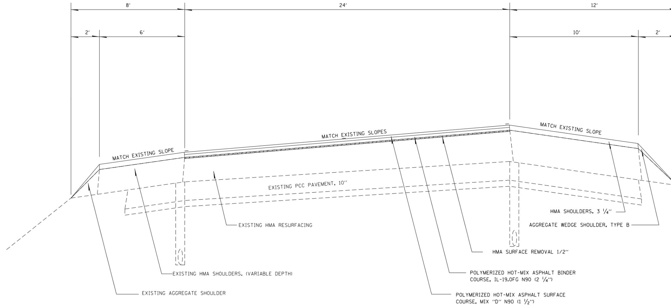
NOTE: THE MAXIMUM ALGEBRAIC DIFFERENCE BETWEEN PAVEMENT SLOPE AND SHOULDER SLOPE SHALL NOT EXCEED 8%.
