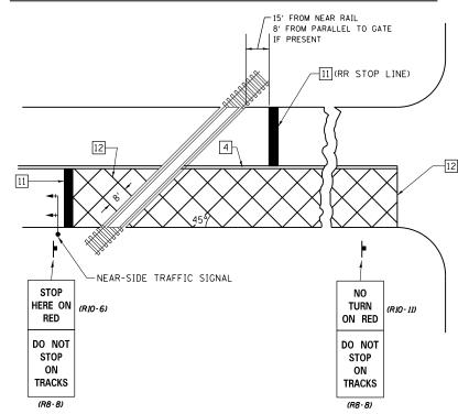
SUPPLEMENTAL PAVEMENT MARKINGS TO BE INSTALLED ONLY ON APPROACHES TO INTERSECTIONS CONTROLLED BY TRAFFIC SIGNALS WHICH ARE INTERCONNECTED WITH THE RAILROAD WARNING SIGNALS.
