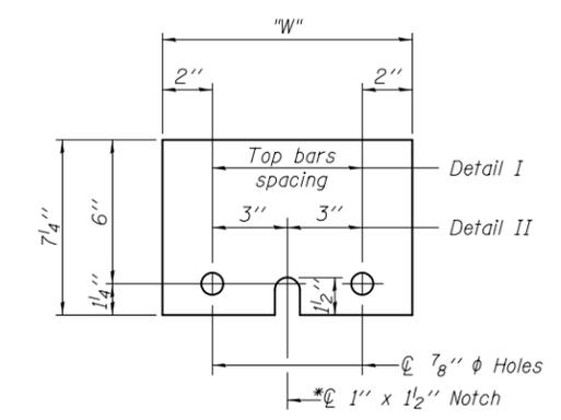
**STEEL RETAINER  $\bar{L}$  1" x 7/4" x "W"**
