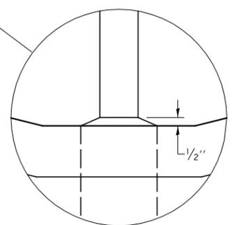
**HIGH TENSION CABLE MEDIAN BARRIER AND WEED CONTROL MOWING STRIP (SPECIAL) DETAIL**
