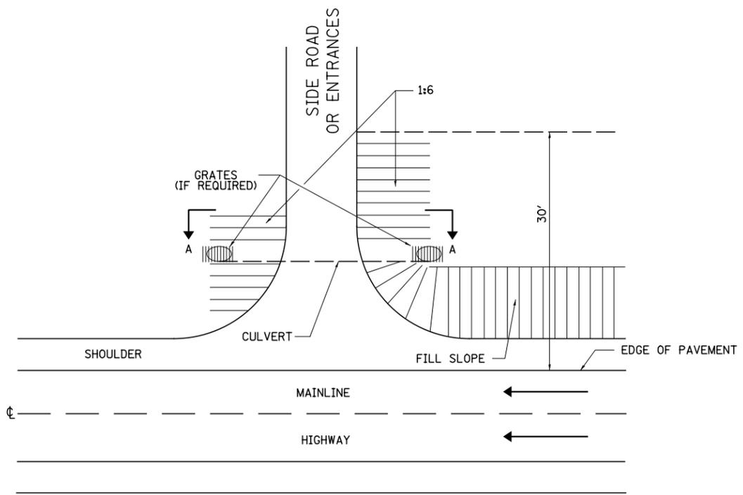
NOTE: ON A ONE-WAY FACILITY, THE GRATE ON THE DEPARTURE END IS NOT REQUIRED.
