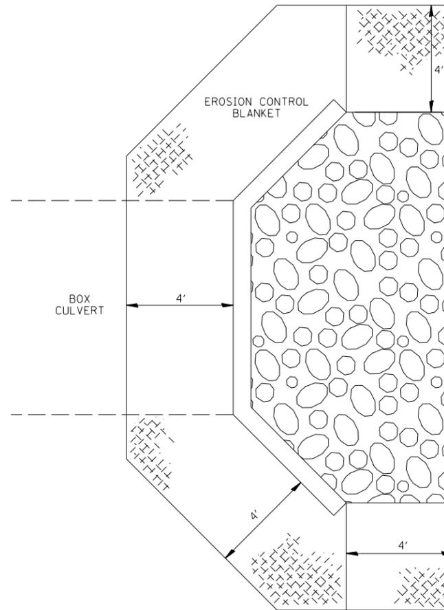
**AT BOX CULVERT END SECTIONS**
