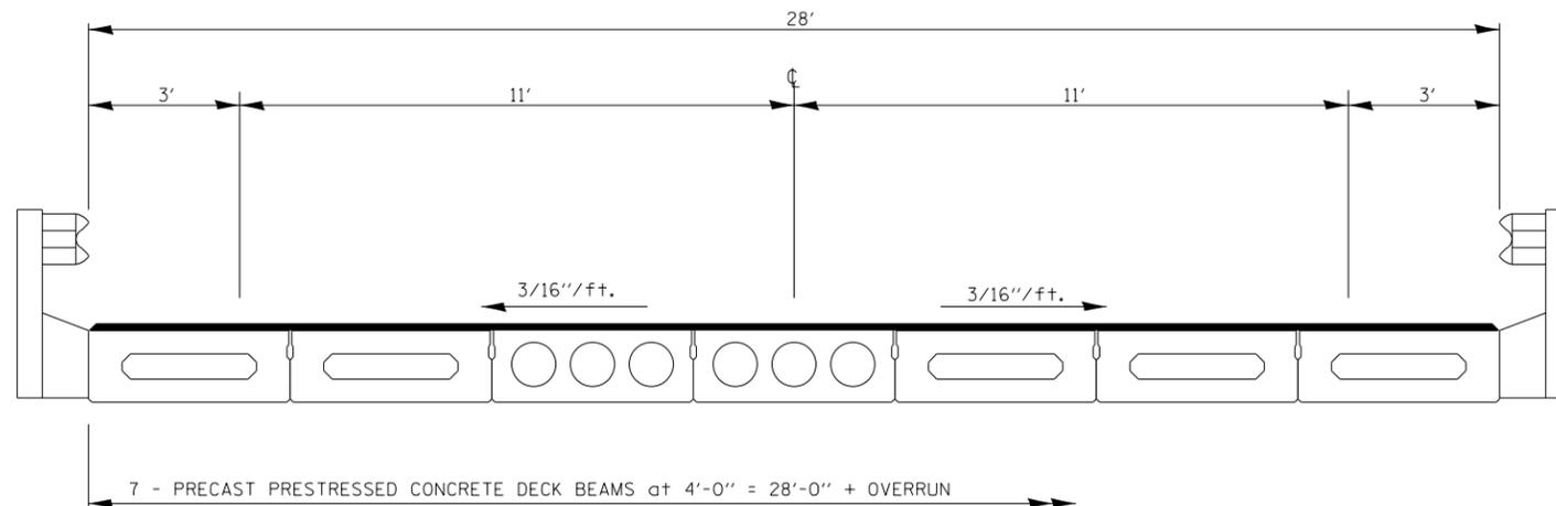
SPAN 2 CROSS SECTION
