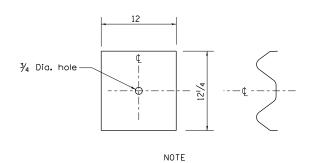
Plate A shall be placed between rail element and block-out at non-splice mounting points only when steel block-outs are used.
