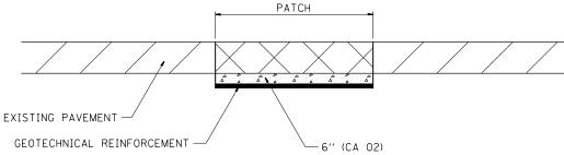
THE CA 02 SHALL BE COMPACTED IN A MANNER APPROVED BY THE ENGINEER, IF THE MOISTURE CONTENT OF THE MATERIAL IS SUCH THAT COMPACTION SATISFACTORY TO THE ENGINEER CANNOT BE OBTAINED, SUFFICIENT WATER SHALL BE ADDED SO THAT SATISFACTORY COMPACTION
