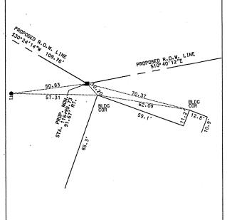
STAKING OF PROPOSED RIGHT OF WAY IN CULTIVATED AREAS. BURIED 5/8 INCH METAL ROD 20 INCHES BELOW GROUND TO MARK FUTURE SURVEY DISK POSITION IDENTIFIED BY COLORED PLASTIC CAP BEARING SURVEYORS REGISTRATION NUMBER. PERMANENT SURVEY MARKER, I.D.O.T. STD. 2135 (TO BE SET BY OTHERS)
