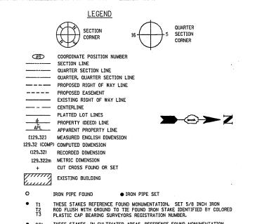
THESE STAKES, IN CULTIVATED AREAS, REFERENCE FOUND MONUMENTATION. BURIED 5/8 INCH 1RON ROD 20 INCHES BELOW GROUND TO TIE TP FOUND IRON STAKE. IDENTIFIED BY COLORED PLASTIC CAP BEARING SURVEYORS REGISTRATION NUMBER.
