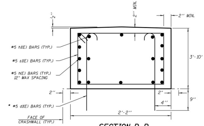
\* EPOXY GROUT BARS IN 9" MIN. HOLES ACCORDING TO ARTICLE 584 OF THE STANDARD SPECIFICATIONS.
