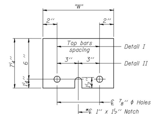
**STEEL RETAINER  $\bar{L}$  1" x 7 1/4" x "W"**
