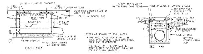
SEE STANDARD 602701 FOR DETAILS OF STEPS. 25 (1) PREFORMED EXPANSION JOINTS AS SHOWN SHALL BE PROVIDED ON EACH SIDE OF INLET.
