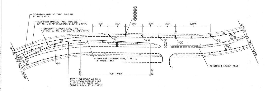
NOTE: PAVEMENT MARKING TAPE, TYPE III MUST BE USED ON THE PAVEMENT OUTSIDE OF THE PROJECT LIMITS IN ALL STACES. FOR STACE III, USE PAVEMENT MARKING TAPE, TYPE III ON THE NEW HMA SURFACE PROIR TO THERMOPLASTIC PAVEMENT MARKINGS.
