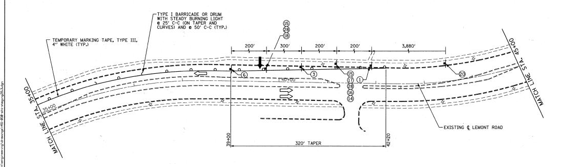
NOTE: 1. THE CONTRACTOR SHALL REMOVE THE EXISTING CURB AND GUTTER, MEDIAN AND EXCAVATE THE LANDSCAPED MEDIANS, AS NEEDED, PRIOR TO PLACING THE TEMPORARY PAVEMENT AS DIRECTED BY THE ENGINEER.
