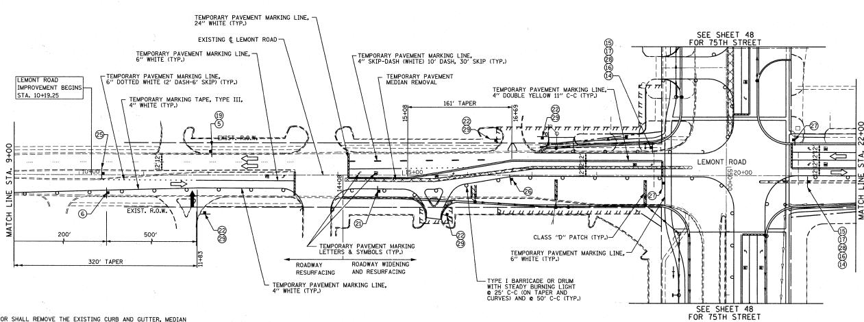
NOTE: 1. THE CONTRACTOR SHALL REMOVE THE EXISTING CURB AND GUTTER, MEDIAN AND EXCAVATE THE LANDSCAPED MEDIANS, AS NEEDED, PRIOR TO PLACING THE TEMPORARY PAVEMENT AS DIRECTED BY THE ENGINEER.
