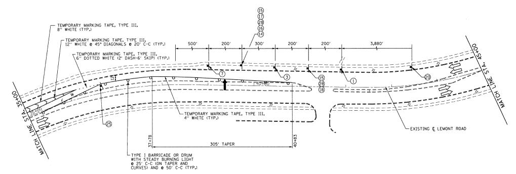
NOTE: PAVEMENT MARKING TAPE, TYPE III MUST BE USED ON THE PAVEMENT OUTSIDE OF THE PROJECT LIMITS IN ALL STAGES. FOR STAGE III, USE PAVEMENT MARKING TAPE, TYPE III ON THE NEW HMA SURFACE PROIR TO THERMOPLASTIC PAVEMENT MARKINGS.
