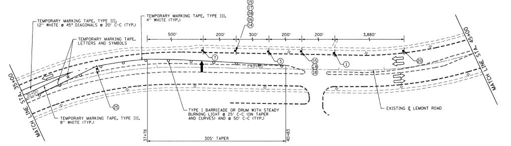
NOTE: 1. THE CONTRACTOR SHALL REMOVE THE EXISTING CURB AND GUTTER, MEDIAN AND EXCAVATE THE LANDSCAPED MEDIANS, AS NEEDED, PRIOR TO PLACING THE TEMPORARY PAVEMENT AS DIRECTED BY THE ENGINEER.
