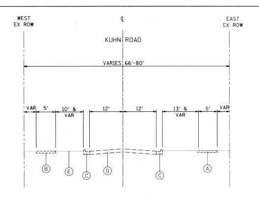
SODDING LIMITS ARE EITHER TO THE PR TEMP EASEMENT, PR ROW, EX ROW, OR 5 FEET OFF EDGE OF PATH, SEE PLAN FOR SODDING LIMITS.
