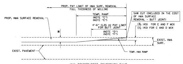
HMA CONSTRUCTED TEMPORARY RAMP
