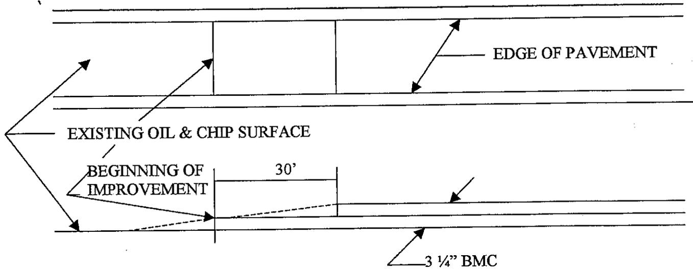
NOTE: PROPOSED TRANSITION TO BE TAPERED AS SHOWN AND ADJUSTED TO MATCH EXISTING SURFACE WITH A CONSTRUCTION JOINT
