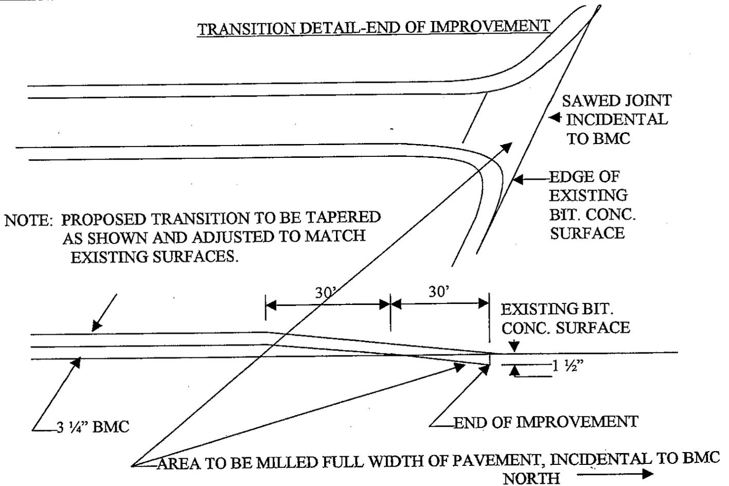
NOTE: PROPOSED TRANSITION TO BE TAPERED AS SHOWN AND ADJUSTED TO MATCH EXISTING SURFACES.
