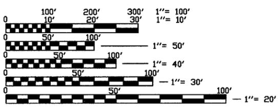
FULL SIZE PLANS HAVE BEEN PREPARED USING STANDARD ARCHITECTURAL SCALES, REDUCED SIZED PLANS WILL NOT CONFORM TO STANDARD SCALES, IN MAKING MEASUREMENTS ON REDUCED PLANS, THE ABOVE SCALES MAY BE USED.
