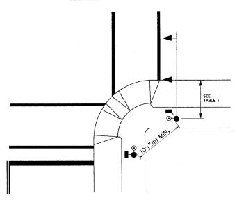
RECOMMENDED PUSHBUTTON LOCATIONS FOR ACCESSIBLE PEDESTRIAN SIGNALS SHALL BE IN ACCORDANCE WITH THE CURRENT MUTCO (SEE NOTE I). TO MEET MUTCO REQUIREMENTS, PEDESTRIAN SIGNAL PUSHBUTTONS MAY HAVE TO BE MOUNTED ON A SEPARATE POST.
