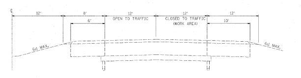
F.A.I. 55/70 SOUTHBOUND STA. 1348+00 TO 1360+00 SHOULDER WIDTHS NARROW UNDER STRUCTURE
