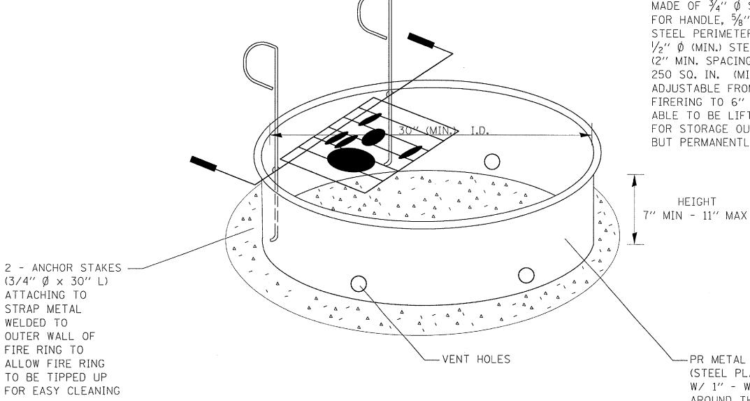
1 - ADJUSTABLE GRILL. MADE OF  $\frac{3}{4}$ "  $\phi$  STEEL BARS, FOR HANDLE,  $\frac{5}{8}$ "  $\phi$  (MIN.) STEEL PERIMETER BARS  $\frac{1}{2}$ "  $\phi$  (MIN.) STEEL GRATE BARS (2" MIN. SPACING) 250 SQ. IN. (MIN.) COOKING AREA, ADJUSTABLE FROM TOP OF FIRERING TO 6" (MIN.) HIGHER. ABLE TO BE LIFTED AND TURNED FOR STORAGE OUTSIDE OF RING BUT PERMANENTLY ATTACHED.
