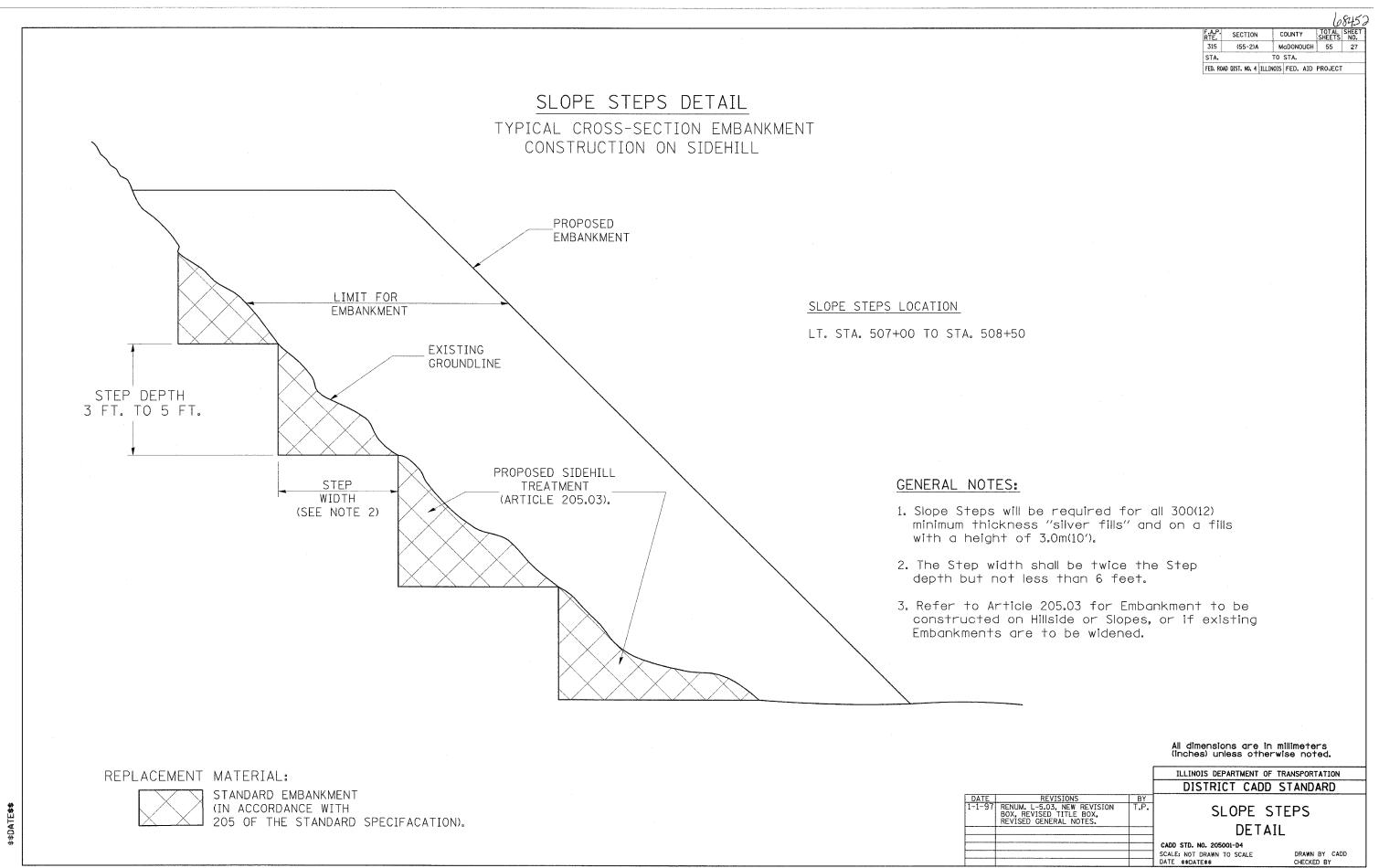
NOTE: EACH PROJECT SHOULD BE REVIEWED INDEPENDENTLY FOR TREATMENT REQUIRED. REFER TO THIS DETAIL WITH NOTE ON APPLICABLE TYPICAL SECTIONS.
