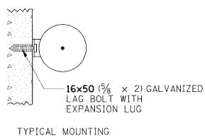
TYPICAL MOUNTING WITH REFLECTOR, BRACKET, & BOLT
