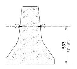
REFLECTOR MOUNTED ON CONCRETE BARRIER
