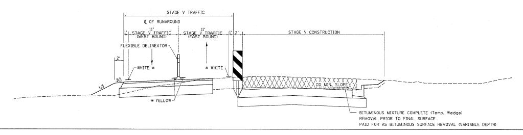
\* ALL PAVEMENT MARKING TAPE IS TYPE III WITH COLOR OF TAPE SHOWN ON TYPICALS SEE SCHEDULE FOR PAINT PAVEMENT MARKING LOCATIONS
