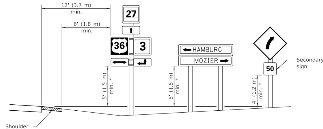
\* In any area where parking is likely to occur or where there are obstructions to view or where signs are located over sidewalks, the height shall be at least 7' (2.1 m).
