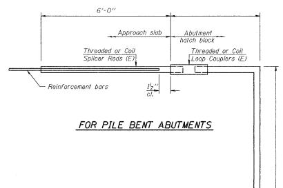
Bar Splicer for #5 bar Min. Capacity = 23.0 kips - tension Min. Pull-out Strength = 9.2 kips - tension No. Required =
