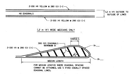
DIAGONAL LINE SPACING; 15 m (50') C-C (LESS THAN 50 km/h (30 MPH))
