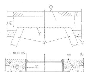
BRICK, MORTAR, OR CONC. ADJUSTING RINGS
